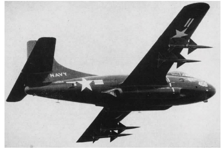
Douglas F3D Skyknight used in development of the Sparrow (later AIM-7) air-to-air missile, 1954
